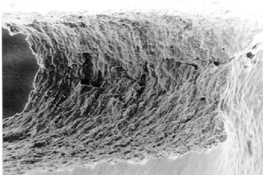
Fig. 10: Blunting before onset of ductile tearing of the crack (acc. to Blumenauer)
