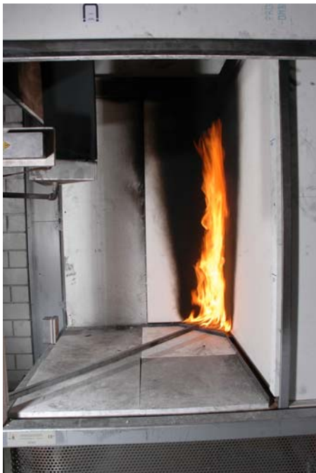
Fig. 3a : MPA Universität Stuttgart fire department test laboratory with SBI–test apparatus
