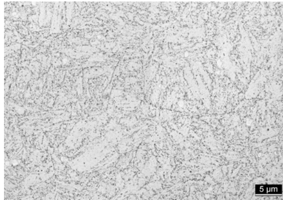
Figure 8 : Montage of four TEM low magnification bright field images of an extraction replica produced from the test material A in the initial state.
