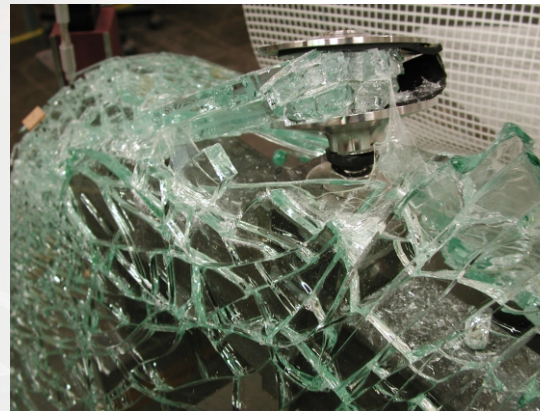
Testing of laminated safety glass and fracture pattern
