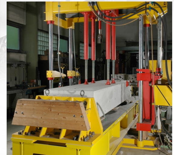
Testing of fastening elements under tension and shear in cracked concrete
