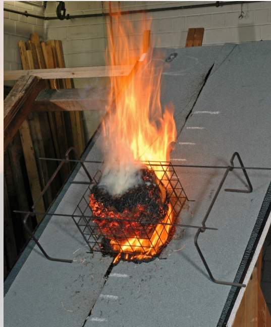
Testing of the fire resistance of roofs against radiant heat and flying brands acc. to DIN 4102-7 and DIN CEN/TS 1187
