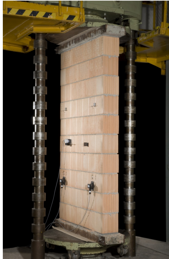
Determination of compressive strength and deformation behavior of masonry
