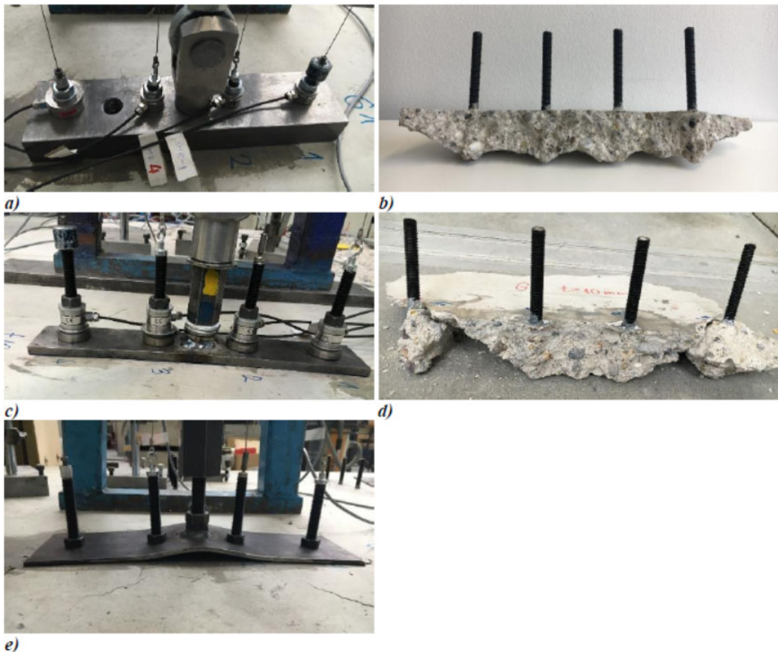
Fig. 2: Influence of the anchor plate thickness (stiffness) on the anchor group a) anchor plate with sufficiently stiff anchor plate G81 ( d = 40\text{mm} ); b) break-out body G81; c) anchor plate with flexible anchor plate G83 ( d = 10\text{mm} ); d) break-out body G83; e) thin anchor plate G84 ( d = 5\text{mm} ) [1]
