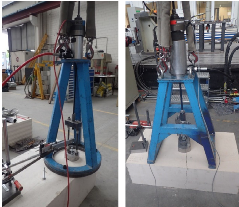
Fig. 1: Unconfined test setup for tests with bonded anchors (left) and with undercut anchors (right) [9]
