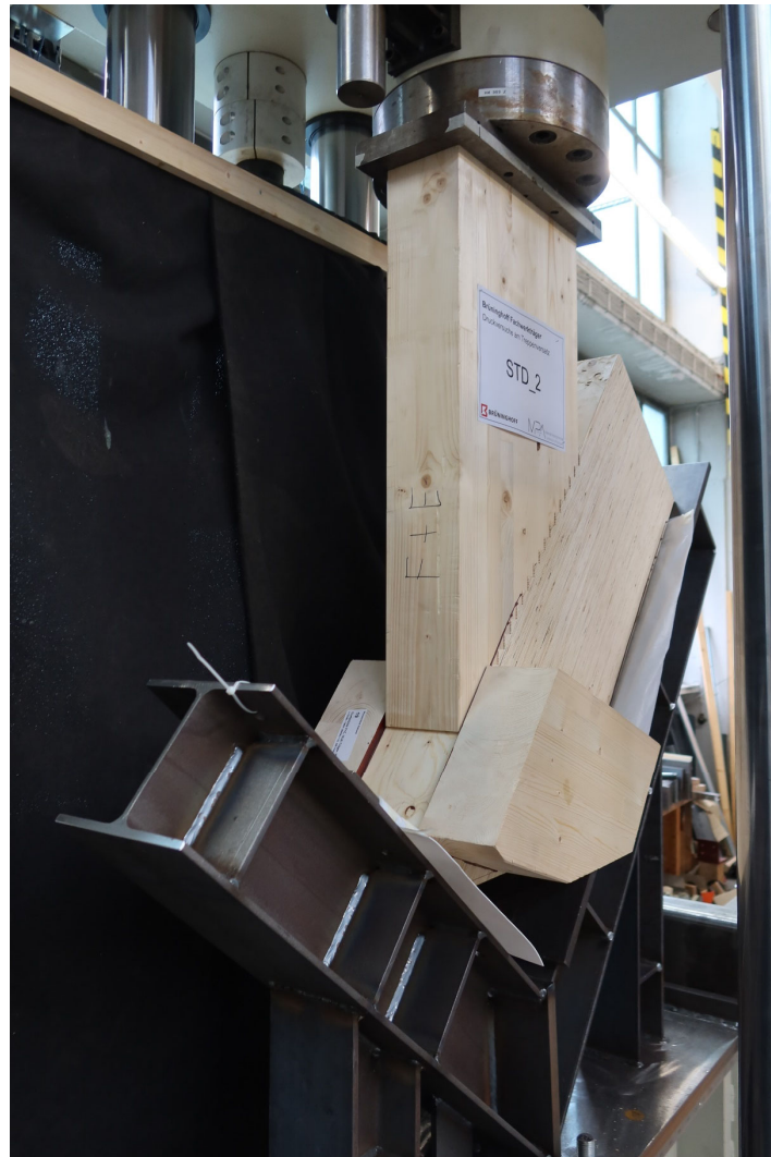
Fig. 6: Realized experimental test setup for the compression-shear test of the contact connection
